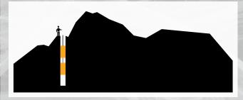
Hydraulic testing and monitoring of defined borehole sections to estimate the hydraulic parameters (steady-state hydraulic head, transmissivity, permeability, storativity, etc.) of geological formations or engineered barriers.
