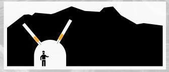
Borehole or borehole section sealing to enable pressure and depth-oriented grouting or injecting for consolidation and waterproofing.
